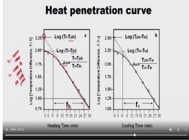
So this is the heating curve as well as cooling curve. So what happens, I will keep my crates and in the retort then I will switch on the steam. So it will take some time to reach the particular sterilization temperature. So that is nothing but come up period then after it reaches the sterilization temperature required temperature, it will be kept at a particular time period. Then the cooling starts, starts in the sense it should come to environmental temperature.
