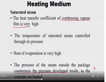
So what are all the heating medium, famous heating medium used is the most famous is saturated steam. So because of the following reasons, one is heat transfer coefficient of the condensing vapor film is high. So that means what happens, so when the heating medium is given into the retort, so after some time, so the condensing vapor forms the film near the packaging.
