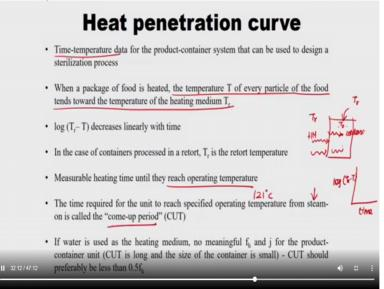
And the important topic of this lecture is this heat penetration curve. So any I would require my time temperature data for the product container system that can be used to design a thermal sterilization process. So what we have seen now, so this is my packaging. So my heat transfer medium is there, so from this heat has to conduct or convect to the packaging material, from the packaging material it would reach the coldest point.
