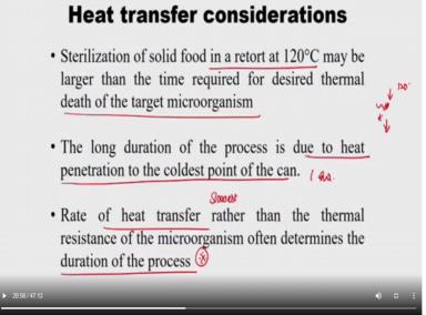
So this thermal gradient causes the thermal stresses, but you are outside your steam will be of high pressure. So this thermal stress is also there which is developed for low thermal conductivity material. So this is this makes unfavorable situation.
