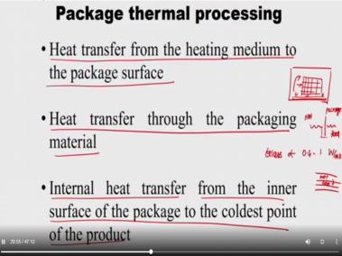
So as I told earlier it is not only the heat transfer medium which transfers heat efficiently, but it also has to pass through the packaging. So if you have a packaging of low thermal conductivity material, for example glass, so the glass the thermal conductivity varies between 0.4 to 1 watt per meter Kelvin. So in such case what happens is there will be thermal gradient in the packaging material.
