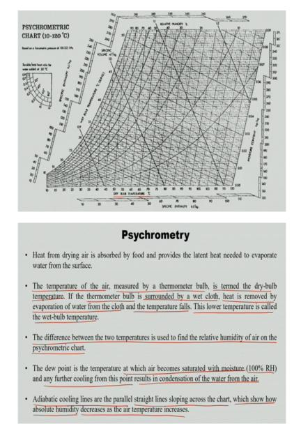
This is the psychrometric chart. So, if you see here in x-axis what you see is the dry bulk temperature right. So what is dry bulb temperature? The temperature of the air, measured by thermometer bulb, is termed as the dry bulb temperature. So what we normally measure at labs. So that is nothing but a dry bulk temperature, which is in degrees centigrade.
