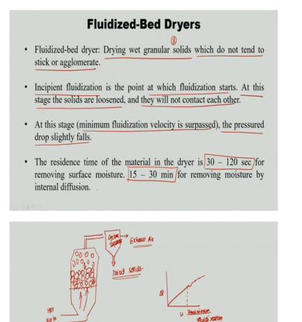
So the next one is fluidized bed dryers, so normally fluidized bed dryer will have a. So this is your air in that means hot air, so you have a perforated plates in which your food particles were kept okay, so this is your exhaust, so this is attached to the cyclone separator from which your exhaust air is coming out.
