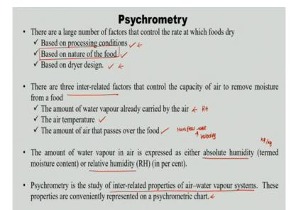
And before going into the main classification of dryers or the various dryers used in the industry, we also should know little bit about psychrometry. I am not going into detail, but because the drying conditions right. In the first slide itself, we have told the drying conditions used is very much important to maintain the nutritional value of the food as well as the food quality right.
