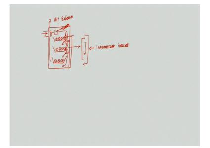
And the next one is tray dryers. So these consist of an insulated cabinet fitted with shallow mash or perforated trays, each of which contains a thin layer of food. So, which is about 2 to 6 centimetre deep right. So one cabinet is there in which a lot of trays, perforated trays in which the food material is kept. So the thickness of the food material here is 2 to 6 centimetre.
