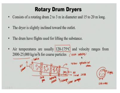
So the next one is rotary drum dryers. So, which consist of a rotating drum 2 to 3 metre in diameter and 15 to 20 metre long right. The dryer is slightly inclined towards the outlet. So it is something of this kind, this is a hollow cylindrical drum. So this is the air exhaust, this is feed in. So you have various provisions here, so here the one is drive gear, then supporting rollers, the third one is discharge screw conveyor.
