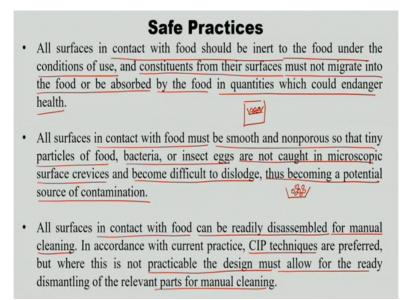
So the safe practices are also being ensured while designing a dryer. So one thing is the surfaces in contact with the food should be inert to the food under the conditions of use, and the constituents from their surface must not migrate into the food or be observed by the food
