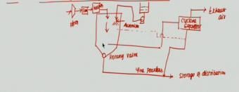
So there is also significant evaporative cooling effect, so that surface temperature of the droplets does not rise much above the wet bulb temperature of the drying air until drying nears the completion. So total drying takes place in the temperature less than the wet bulb temperature of the drying air. Because the particles are the droplets does not increase the temperature right.
