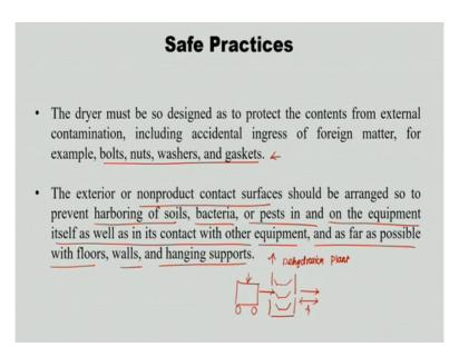
The dryer must be so designed as to protect the contents from the external contamination, including accidental ingress of foreign matter, for example, bolts, nuts, washers, gaskets. So this also should be contamination free because these are all the small components which are used in the dryers. It is not only the drying surface. The bolts, nuts, washers, gaskets are also should be contamination free.
