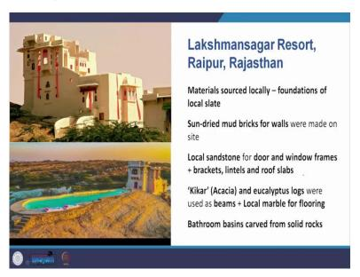
For example, her project is the Lakshmansagar Resort in Raipur Rajastan where the materials were sourced locally, so the foundation. The entire project has this aspects in it, the foundation is in local state. Sun-dried mud bricks for the walls. Local sandstone for the doors and window frames. So, the bracket, lintels and roof slabs. Kikar or Acacia wood and eucalyptus logs for the beams, local marble for the flooring and the bathroom basins have been hewn out of solid rocks.
