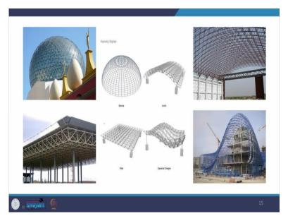
So, here we have the various types of space frames that are visible around us today. There is the geodesic dome, and this is a vault in space frame is a flat roof in space frame. This is an example that you can find in a center that was designed I believe, by Norman Foster in England, and then you have the Heydar Aliyev center with a curvy linear firm that is possible because of the space frame.
