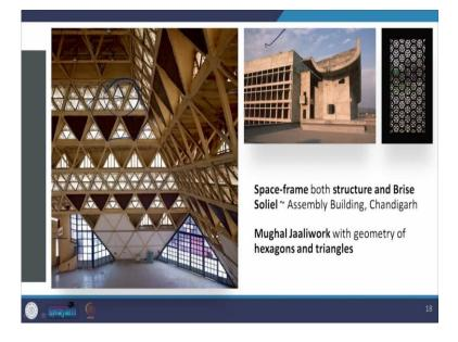
Now, in this case, the spaceframe of the Pragati Maidan or Raj Rewal pointed out that this happened to be both the structure and the sun breaker or the brise soliel. In the case of Corbusier's building like the Assembly Building in Chandigarh, the structure was separate and the brise soliel was mounted on the building. So, the brise soliel was not a part of the structural system.
