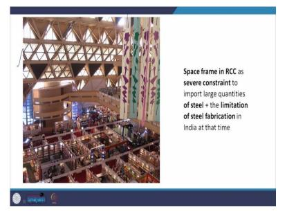
And this is a picture that shows you how amazingly this space can be used, there are a series of exhibition spaces that are housed here within the Hall of nations and the even the height becomes useful. So, the space frame was an RCC because of the severe constraint or of importing large quantities of quality steel to manufacture it in India, along with the limitation of steel fabrication at that time in India.
