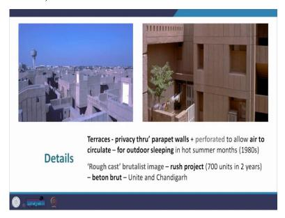
So, details that is terraces are there are privacy is through the parapet walls. The parapet walls are perforated to allow air to circulate as people are sleeping on the beds. So, through the parapet perforations the air would flow in and it would become a stronger breeze because it is going through smaller apertures. And therefore outdoor sleeping in hot summer months becomes a pleasant exercise, a pleasant endeavor.
