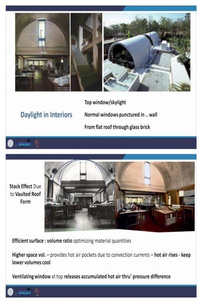
So the daylighting in the interiors is diffused. It pulls in from the skylights that are there in the barrel vault. And even there is a full window here. If you just go back you see the full window here. It is pulling in the light and the normal windows, they are punctured into the wall. And there is also this flat roof in which there are these glass bricks provided and light filters in through this also. And over these glass bricks the following water is passing.
