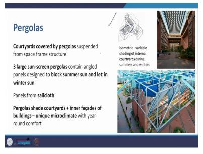
And the pergolas. The courtyards are covered by a pergolas suspended through a space frame structure. So, the idea is coming from earlier, but now the technology being used is a modern technology. There are three large sunscreen pergolas that contain these panels which are angled and they block the summer sun and let in the winter sun and the panels are made of sailcloth.
