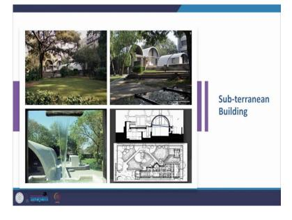
So this is a subterranean building. As you can see, this is the section and part of the building this much, it is underneath, it is cut into the earth, earth on both sides, and the barrel vault is on the outside.
