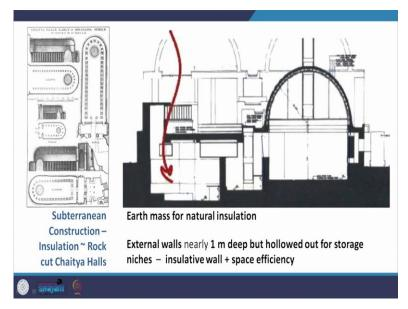
When we talk of the subterranean structure we are also reminded of the Chaitya halls and the rock cut chaitya halls. And here we have it. Because of the earth mass on either side it creates natural insulation. But they have taken advantage of these thick external walls which are nearly one meter deep by hollowing them out and creating storage niches in them. So it is insulating, as well as there is space efficiency through that.
