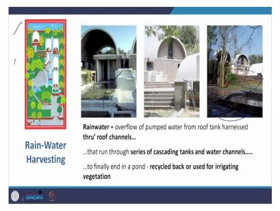
Now rainwater harvesting in cycle. This of course, is a classic example of B. V. Doshi making the drawing of the building as a Rajasthani painting. As you can see it lacks perspective, it does not have the feeling of depth in it, it is flattened out as it would be in Rajasthani painting.
