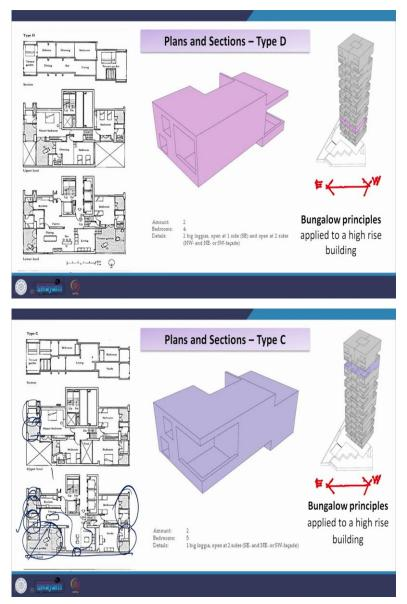
He does that in type C, he does that in type D, he is trying to keep the living spaces as protected as possible from the direct impact either of the monsoon rains, or the glare of the sun.
