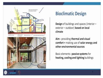
Now, what is bioclimatic design? That design of buildings spaces that is based on the local climate and the aim is to provide thermal and visual comfort by plus making use of solar energy and other environmental sources. So, if I were to take a section of a bioclimatic house, it would have the breeze flowing in through and through it would have the use of the sunlight, use of proper shading devices et cetera etcetera.
