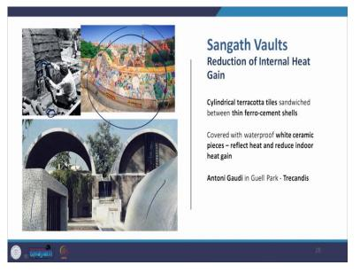
And then there is the reduction of the internal heat gain. Now, if you watch very carefully this picture, this barrel vault that is being created in the barrel vault, there is one layer beneath
