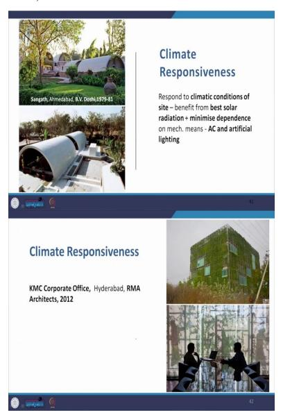
Climate responsiveness we find, for example, in Sanghat, with the barrel walls that have been covered with broken ceramic tiles, to reflect back the solar radiation, respond to the climatic conditions of the site, benefit from the best solar radiation, minimize dependence on mechanical that means air conditioning and artificial lighting.
