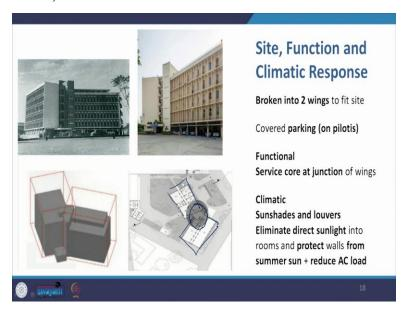
Now, with regard to the site function, climatic response, the entire building, the UGC building is divided up into two wings, to fit into the site and it has covered parking. The parking is provided by raising the building on a Pilotis. And the functional part that we see here is the Service Core is at the junction of these two wings of the UGC building. And then there are the sunshades and louvers provided.
