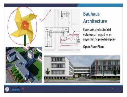
Now the basic structure is logically thought out system of connecting wings corresponding to the internal operation of the school and here it is flat slabs and cuboidal volumes as I mentioned earlier arranged in an asymmetrical pinwheel plan. It's a pinwheel plan as you can see here, it is a pinwheel organization.
