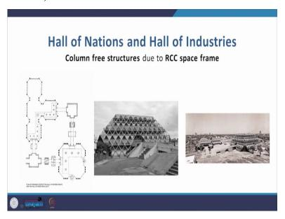
But you can see that it is an idea, now the built form of Hall of Nations, you do not find anything like that in Corbusier's work. This is a space frame but the only thing is, it is an exposed RCC. Now it is column free structure because the space frame is carrying the load. So, massive open spaces are created due to the RCC space frame in the Hall of Nations and the connected hall of industries. You see the entire complex in this picture.
