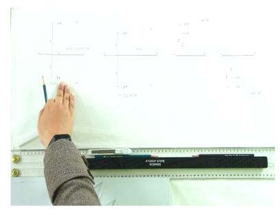
So, the first thing that we have to draw is a reference line. This is the reference line the XY line. Now when we are drawing the projections in first quadrant we know very clearly that the top view or the plan is going to be seen below the reference line and the elevation is going to be seen above the reference line. Now, visualize it again we have this point here which is at 5 centimeters from the VP.
