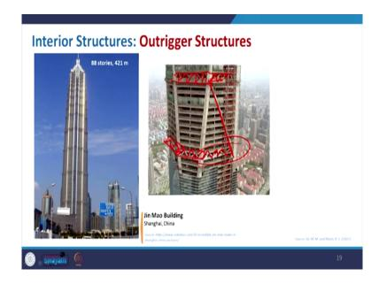
Now, this is another example for this is Jin Mao Building in China, here you can easily see this is the finished product, but here you can see that how this floor being managed. So, here also you can get some bracing structural bracing that being made and also in this floor it is basically giving this truss which is made of concrete and then it is giving this particular belt truss.
