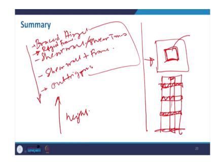
So, this is all about the interior structure where we have seen this. So, if we just try to summarize we have the braced hinge structure and then we have the shear wall then also we have seen the shear wall or shear truss is the same. And we can use a concrete or steel to make this then you have your shear wall and then your frame interaction.
