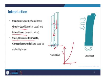
So, here you can see that all the date load of the building and all they are acting axially and they are transferring to the foundation and foundation will have a reaction. So, this is very common for all the buildings and even for once for the building as well. But, at the same time when you think of increasing height as because with the increase the lateral movement of a building will be more due to the wind pressure.
