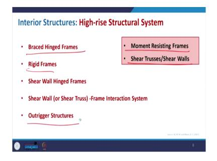
So, if I move forward, so basically for any structures structural system, two important parameters are there. One is your moment resisting frames which will resist the moment due to the lateral load and the other one is your shear truss and shear wall. So, these two components these two components they are playing the crucial role in any structural system. When you combine both of them together it will give you better result and we will see that how that can be combined.
