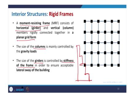
So, here it basically a moment resisting frame that consists of the horizontal girder and vertical column, so they are actually linked fixed rigidly and they are co planar. So, it is basically a linking then this you know very typical grid structure. The size of the column is mainly controlled by the gravity load that already I explained to you. That whatever the axial vertical
