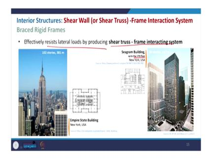
So, in this case if you see, this is the braced rigid frames where effectively resist the lateral load by producing shear truss frame interacting system, it is common for both. And this is example for Empire State Building in New York. And here also it is the Seagram Building both are very commonly used building examples in architecture there this system being used; moving forward the shear wall rigid frames.
