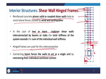
Now, coming to the shear wall hinge frame where it is not the connection, all the connection being made with only the column and the girders. So, here in state of that at the core as interior structure that we are discussing now, we use the shear wall. So, shear wall is basically is maybe the RCC wall which will act as basically as a cantilever to the base, so it can sway. So, other structure is holding it is giving the support, so main lateral force the this being resist by this core.
