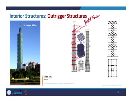
Coming to the example this is a the example of Taipei, so here you can see that in different levels, in the section though it is not much clear, but you can see some of the places where this being used at different you know interval. So, along with the core truss that we have, so also we have this kind of truss system this is also called belt truss.
