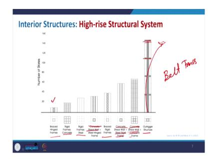
So, if you see that here in the y axis it is given as a number of storey the number of floors you may say a standard floor, and here is basically the improvement of structural element. So, when you go with the braced hinge frame you cannot really go much because of the hinge condition where it will again have some you know flexibility it will allow some rotation and bending and all.
