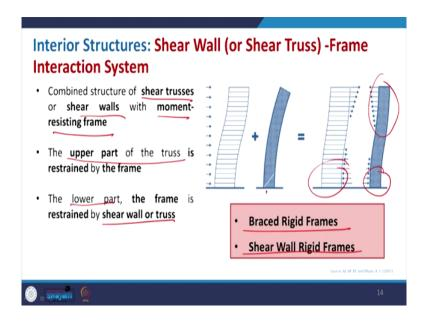
So, I would suggest that you go through you will get more information about that how it works. Now, coming to the interaction, yes. So, here it is basically where you just use your frame moment resistance frame, so it will have a movement and then this is basically the shear truss or shear wall and then when you combine. So, the combination of shear truss and shear walls with moment resistance frame.
