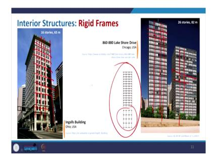
Now, coming to the rigid frame structure, here are two examples and here it is a typical plan where you can see typical plan and elevation where the beam your you know the girders and the columns being actually compiled. So, in this case if you see that this is your Ingalls Building in US there is 16 storey's 65 buildings. So, here it is a very simple structure. If you just see from the exterior, so their vertical members like this and then it is been connected.
