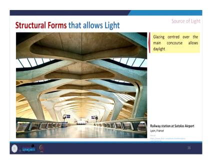
So, in this case you can see that the structure is nothing but a frame again, but this time it is made of concrete or the steel and this is designed in such a manner that the place the gap between these two portal is being covered with glass and that is giving the enough light to you know luminate this concourse level.
