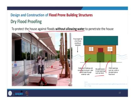
So, this flood panel will protect that direct thrust of the flood water towards that building and even here you can see like the doors and other thing is being protected with a movable shield, which will be removed when the flood level reduced and then the risk will be no reduce or that will be lower down.
