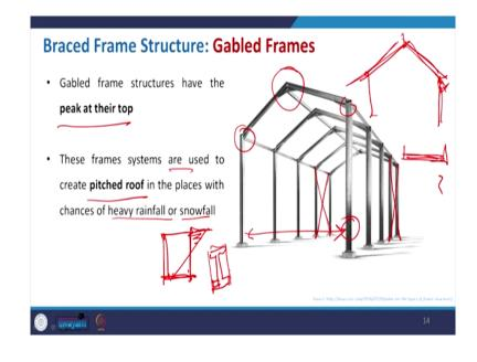
So, the member this particular frame we have little bit height. So, gable frame structure have a peak at their top. So, here you can see that how it is connected and at the same time in order to protect it from the lateral force, you can identify here easily that these are actually braced
