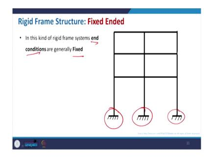
And come to the fixed ended. So, here you can see that the particular representation of the structure has changed. So, now, it is shown like it is fixed end. So, in this kind of rigid frame system, end condition are generally fixed not the pin one.
