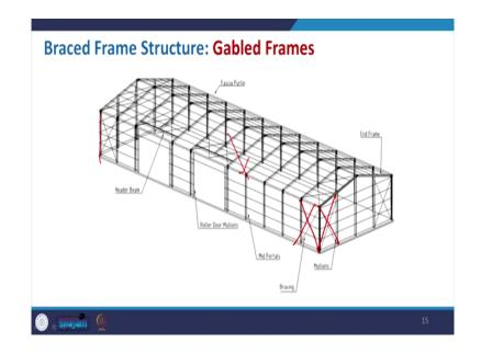
Now, this is something which you can see that it is mostly being used this kind of frame for the manufacturing unit some of the factory. Then it is a very regular arrangement. So, multiple frames are put in parallel and then that will be covered by some light material or some times maybe some translucent material. So, that you know they can maximize the daylight uses inside it and along with that we are also have the bracing to protect the structure the frame from the lateral load.
