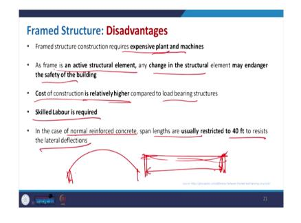
Now, come to the disadvantages of frame structure. So, frame structure definitely requires some expensive plant and machines because whenever you go for higher height. So, you need some other equipment machine to bring your material at upper storey. So, different cranes different leaves.
