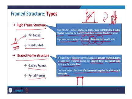
Now, coming to the framed structure that type: so, basically based on the joint how they are actually combined together, how they are connected to the footing. Based on that we have majorly rigid frame structure and braced frame structures. So, bracing here the braced frames come from the bracing that we earlier discussed also like in order to overcome or resist to the lateral load like wind load and all sometimes, we connect your frame with some diagonal member.
