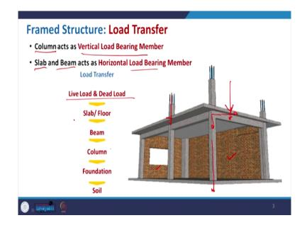
So, here if you see typical schematic of the frame structure though I have shown you the wall, but these are not the load bearing walls. So, they are just used to protect your interior from the outside environment. So, basically the loads imposed on that the dead load, live load; all kind of loads is transfer from your beam to column. So, say for example, this is the slab I just put some load on it. So, this will be transferred to the beam first, then beam will transfer to the
