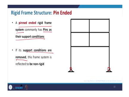
Now, come to the pin ended joint rigid frame structure. So, a pin ended rigid frame system commonly has pin as their support condition. So, here if you see that in this portion and they are joined with this. If this support pin is removed so, that will be considered at non rigid. So, the support condition removed means it will be non rigid structure.
