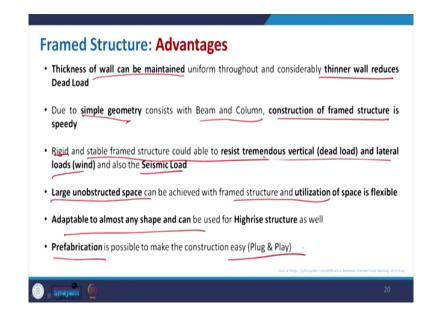
First of all compare to the load bearing structure. Now, the thickness of wall can be maintained uniformly throughout because like thickness of wall will not essentially matter the load distribution because load will be taken care of by the beam column and footing the walls are just to make the partition. So, that can be there and it can be an as a result that can also be thinner compared to your load bearing structure.
