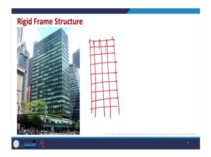
The same kind of thing like when you not go for this kind of you know hotel buildings in Burj Al Arab or so. So, this kind of office towers being also be constructed with the frame structure where it is very simple form that straight you know frame. So, the combination of your beam and column is making the whole skeleton and we can actually use the space more efficiently.
