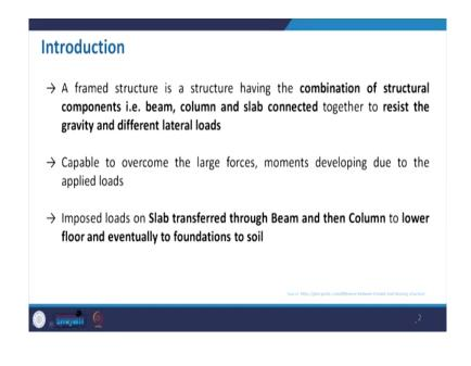
So, let us start this discussion on framed structure. Now framed structure what it says like a frame structure is a structure having combination of structural components like beam, column and slab connected together to resist against the gravity load which is basically also referred as the actual load you know which is acting vertically like transferring from slab to beam, beam to column and then column to foundation and to soil.
