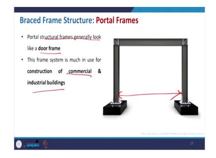
Now, come to the portal frames like instead of the gable now the portal frames that will have a very rectangular section. So, you can identify the portal structural frames generally look like a door frame ok. So, it can also create some you know space. So, it is also being used in some commercial and industrial building where the frames being used.
