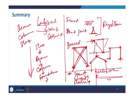
Now, coming to the summary section of this frame structure so, basically in the frame structure is a combination of your beam and column and slab. So, they are being connected to each other which will resist the axial load or the gravity load which is transferring from your slab to beam and then beam to column and then column to your foundation and foundation to soil.
