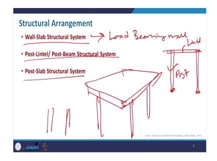
Now, again I am as we know the component with combination and permutation. We can say about three basic structural arrangement start with the wall slab where there is no role of column and specially, it refer to you are traditional load bearing wall. And, still we invented those you know the concrete and the, you know concept of the frame structure and other thing. So, most of the buildings in history we have seen that it is basically the wall slab kind of structure which is load bearing again.
