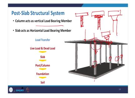
Now, come to the third category, in this case as I mentioned there will be no lintel on something like this particular bend. So, here it is a multiple column placing here and on just top of it this is been placed. And, in this case all these columns that we place here that will take the vertical load or vertical load bearing member where this slab is basically the horizontal one. It will again transfer the load and it will transfer load to the post and column and then foundation through soil.
