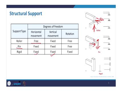
Now, in this case again if you see this the structural support, there a different way we can fix it up one is of the roller type. So, roller type support, we can see in this that one end of the structure will be resting on a roller and normally this structure being used for a bridge. So, that you know during this particular you know movement the oscillation that can roll over it and it can transfer.
