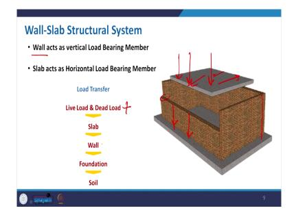
Now, come to the wall slab structural system, again this is a very representative you know structure and this is just for showing you the purpose that here you can you are not able to find out any you know column or something like that is full wall. And the, for the load bearing kind of structures definitely the thickness of the wall at the corner or wherever we go for you know some kind of you know connection.
