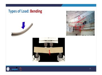
The bending again it is very clear and this is you know laboratory tests where load being applied on a wooden beam and you can see the deformation and cracks developed here. Now in this case again let us understand this with this is the bar and we put pressure from that. So, it will have a sag. So, sagging moment been created, but interesting fact is that, so at the top portion of that ok. So, it is shortened so, as bending said that one end elongate and one end shortened.
