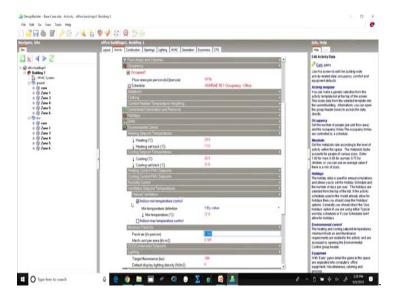
For ventilation set point it will come into picture only when the natural ventilation has been enabled. In this case we are taking an air conditioned building fully air conditioned and when we will move on to the HVAC template, then we will see that whatever value we define here will really not make much of a difference or it will not make any difference, simply because the building has been assumed to be an air conditioned building.
