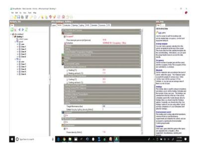
Same as for lighting, so here the target luminance has been taken as 300 lux which is what NBC also defines. So, 300 lux for an office building is the default target luminance.
