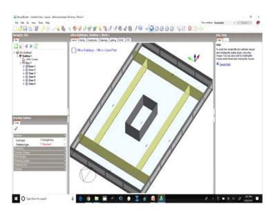
Now, when we have created these virtual partitions, these virtual partitions do not really physically divide the space into different zones. But, it will only account for the heat exchanges, the difference in heat exchanges and the light which is coming by making it a different partition.
