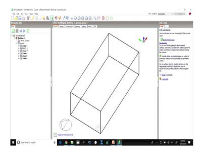
So, this is the core zone. So, we can change this core zone as a core, because this is where our different systems would be. So, this is going to remain an unconditioned space while rest of this area is going to be a conditioned area. So, rest of the zones are basically single zone, but just virtually partitioned. So, this is at the block level.
