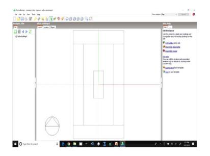
So, suppose we want to organize the DXF in a horizontal manner. So, then in that case we go to Edit the DXF and we can then select 2 points and we can rotate the DXF whichever way we want. So, sometimes the building may not be a very uniform, rectangular, rectilinear building it may have different shapes. So, we may want to orient or rotate the building accordingly.
