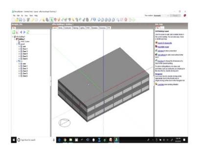
So, all the properties that were there for the ground floor have been copied onto a first floor which is this.
