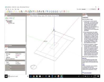
Now, we have to create the Building Block, walls have to be created here we will check the geometry, the Height default height which has been taken as 3.5. In case the building height was more or less suppose you are creating a residential building and you want 3.0 meter height or 2.9 meter height it can be changed from this point.
