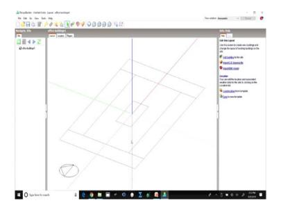
Now, you can see that a very simple single line drawing of this building has been created here, the orientation that it takes is by default. So, in one we are doing the base case as per appendix G, we will have to create the same building and rotate it for 4 different orientations.
