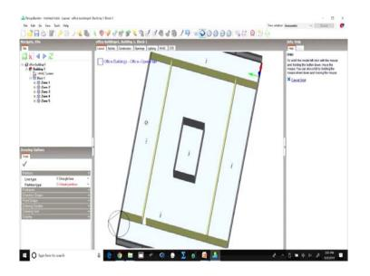
So, we can see that automatically wherever an enclosed zone was created using standard partition or virtual partition the zones have been created. However, because the partitions were not joining, this entire zone is currently behaving as a single zone.
