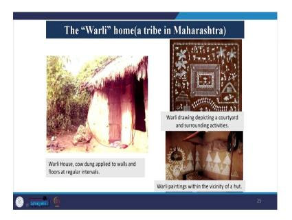
So, we can see these typical designs coming up and again like most of the temporary architecture the Kaccha architecture that we have been seeing, it gets repainted on top every subsequent year after the rains. So, mud and cow dung is applied to the walls after regular intervals at least once a year and the walls are painted and repainted again. So, it only strengthens the wall.
