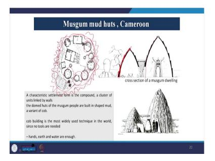
So, what they this people do is, if you look at the design of these huts it is quite similar to some of the huts which we have just seen which are made out of thatch also the plan. So, to optimize the amount of resource the plan is circular which is the most optimized shape. So, minimum surface area which is what was required we have seen Bhoongas also doing the same.
