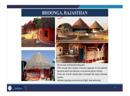
Next we have this example of Bhoonga of Rajasthan; I am sure most of you have already heard of how Bhoongas are designed. So, Bhoonga of Rajasthan are kutcha construction they are not permanent houses yet majority of the Bhoongas have survived for centuries continuously that is by virtue of its design and the optimized amount of resource that it consumes.
