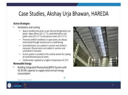
In active strategies they placed a lot of importance on ventilation and cooling. So, the entire space was divided into 3 distinct zones. And the first strategy that they used was maintaining proper set point temperatures as we have seen. So, at 25 degrees plus minus 1 degree in the apex offices and controlled offices and public areas were maintained at 25 plus 3 degree centigrade and passive zones were maintained at 25 plus minus 5 degree centigrade.
