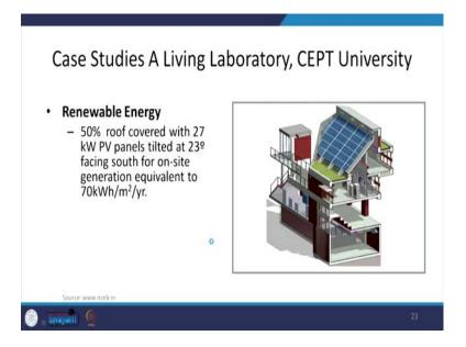
Once this passive and active strategies were incorporated into the building and the EPI was reduced to 58 kilo Watt hour per meter square per year renewable energy was further added where the 50 percent of roof was covered with these photovoltaic panels and they were able to generate the equivalent amount of energy which was consumed in the building thereby making this entire building as a net zero energy building.
