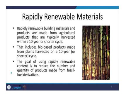
So, what is a rapidly renewable material? It is a building material which is made from agricultural products that are typically harvested within a 10 year or shorter cycle. So, wood which is produced from hard grown timber which takes around 20 to 25 years to fully grow does not come into rapidly renewable material though it is renewable, but it is not rapidly renewable.
