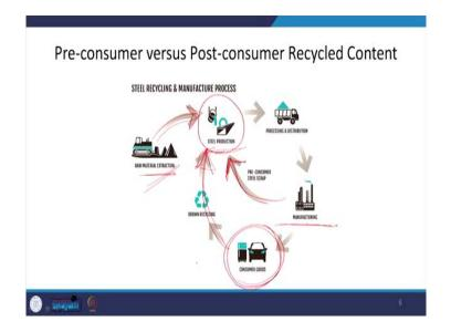
Now, these contents the post consumer and also the pre consumer recycled content would be added back into the manufacturing system. For example, here we're taking an example of the steel production. So, there is raw material which goes into the manufacturing of steel, processing distribution goes into manufacturing and then it is going to the consumers.
