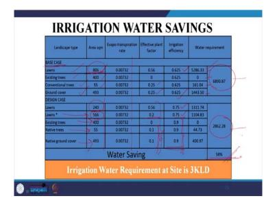
So, once we have all these we will actually put them in the same equation which we just saw and calculated the total irrigation water requirement. One of such calculations is shown here and so, suppose as a base case in the initial stages of the design. We proposed 806 square meter of lawns, 400 square meter of existing trees were retained and conventional trees were planned as 55 square meter of area and there was a grand ground cover which was proposed.
