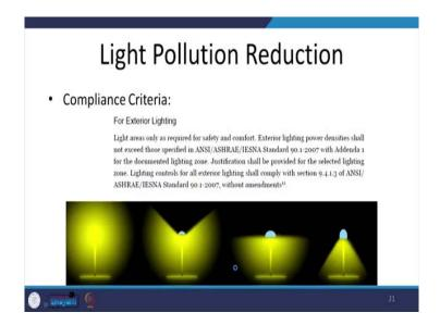
The next one is for exterior lighting. Now, here it directly refers to the codes. We have Indian codes also in practice, ECBC also mentions the lighting power density. So, ensuring that the minimum lighting power density is provided for. So, no extra lighting power density has to be provided.
