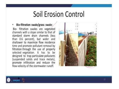
Besides infiltration trench, we have bio filtration swale or grass swale.
