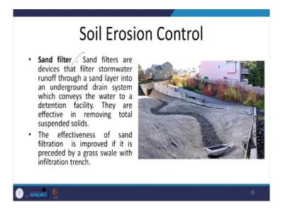
The other is a sand filter. So, sand filters are devices that filter stormwater runoff through a sand layer into an underground drain system. Now here what we are doing is, we are mainly lining the entire channel of this stormwater with sand, which will help to filter, which will help to reduce the speed, and also help in percolation of water down to the ground; and during the process of this filtration, the soil is held back by the sand.
