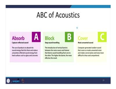
To conclude it all we can say there are 3 fundamental ways in which acoustics of a place of a space can be designed that is ABC absorb, block and cover. So, first is to capture the reflected sound by using appropriate material absorptive material. Second is to block the sound from traveling by introducing the vertical barriers the barriers to this sound which can be possibly disturbing and. The third is to cover the unwanted sound to mask that sound by providing certain covers.
