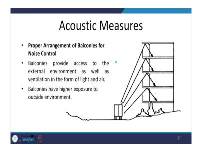
For <u>example\_xample</u>, designing the balconies such a way that is known direct noises hitting into the space it is coming into the space.
