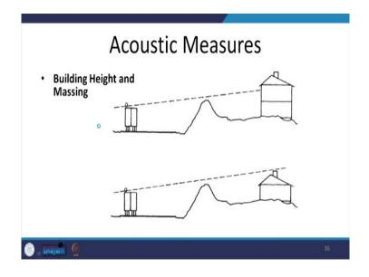
But it is a very thick wall and we should also see that it is porous and that is what causes a lot of sound reduction to happen through this wall. There are other design measures for example, adjusting the building height depending upon the topography and the site features which are available.
