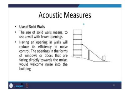
There are multiple other measures for example, using walls, solid walls as acoustic measures. So, this is a highway going and this actually acts as an acoustic measure besides was trees can also act as acoustic measure.
