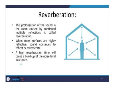
So, reverberation is prolongation of the sound in the room caused by continued multiple reflections which is what we would see in case of different shapes. So, it gets reflected from one surface goes onto the other surface and then further reflected and comes back. So, it will happen only when we have hard surfaces and there are multiple reflective surfaces present in any room.
