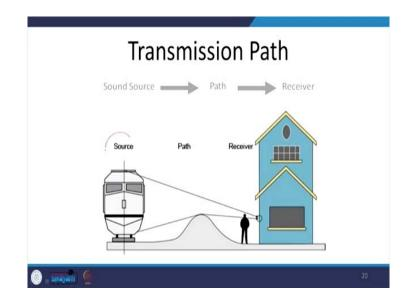
For example, the theaters they require more sound acoustic treatment to provide for the sound quality. So, when we are looking at the design of buildings for acoustic <u>comfortcomfort</u>, we should look at the transmission path we should identify the source, we should identify the receiver and we should look at how what the path of this sound travel is from source to the receiver.
