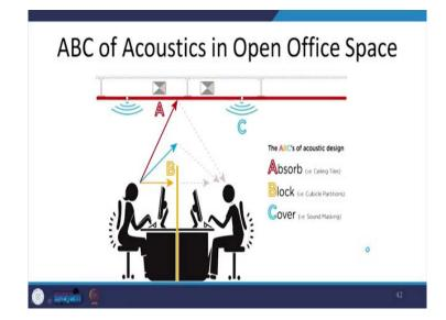
So, when we are looking at strategies in an open office space we are again looking at the ABC we are looking at the ceiling material which is reflect, which is absorptive we are looking at the partitions which block, we are looking at the masking of the sound through provisions of absorptive material here.
