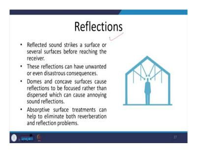
Now, reflection results in reverberation. So, how the sound is going to be reflected? So, it depends upon the material as well as design. So, how the sound is going to be reflected? How many times will it be reflected will result in reverberations. So, for any good classroom or office a reverberation time of around 1.5 is a good reverberation time and we should choose materials effectively.
