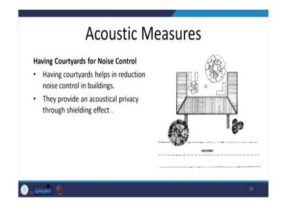
Having courtyards for noise control, so, for example, in this building the courtyard is facing away from the highway and this side would be a blocked side. So, the sound because its travels straight. So, there will be less of sound which will be available in this courtyard.
