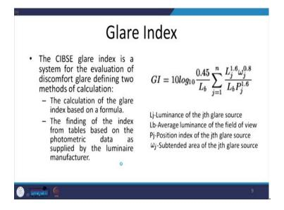
So, to define glare the glare index has been defined which is what we just saw when we were defining the illumination level and the glare indices. So, the formula inn-corporates largely the luminance of the glare source which is under question, the average luminance of the field of view to which the eyes have adjusted, the position index of the glare source how far or how close it is to the object to the area under study subject under study and the subtended area of the glare source.
