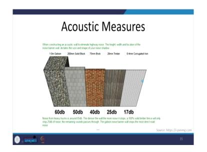
If you are looking at <u>materialsmaterials</u>, we should understand the difference between each material and the amount of sound reduction, insulation that each of these materials provide. So, the walls the regular walls provide around 40 Decibel of a sound insulation difference from the source to the sink side. If you want around 60 Decibel around 1 meter of Gabion is a useful strategy or useful material.
