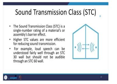
Lower is that number the better is this material for sound insulation the same is further taken to understand or classify the materials in different classes. So, there are, there are sound transmission class STC. So, higher this STC values are the more efficient is the material for reducing sound transmission. So, it is an inverse of NRC in a way.
