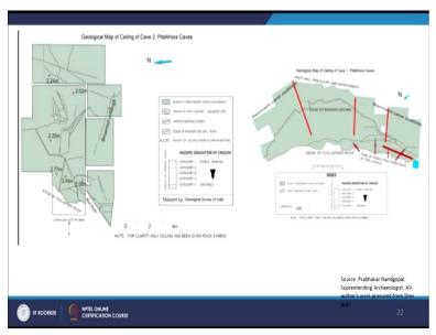
One is the slightly weathered vesicular basalt and also water seepage zones which are more of this dotted aspects of it and where the edge of the broken ceiling you know the roof, and this is where they try to again classify all these aspects and also where the cracks are also appearing continuously not only in a horizontal in the ceiling level but throughout the cave structure, how this vertical cracks are also coming up.
