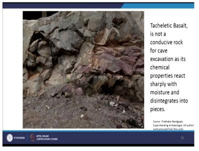
And this Tacheletic Basalt which is not a conducive rock for cave excavation as its chemical properties react sharply with moisture and disintegrate into pieces. The moment you are making an excavation process, it gradually brokes into small wedge-shaped pieces you know, that is one of the important aspect in the excavation challenges and excavation challenge especially with this kind of material.
