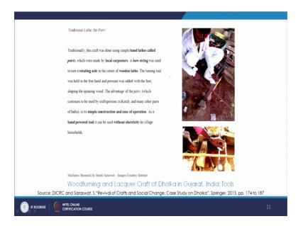
So, if we seen another craft cluster in one of the other villages of Gujarat the traditional lathe which is called as patris used and this work is entirely done by hand; so it is a very simple mechanism. It has an easy operation, it works without electricity and it works as a hand powered tool.
