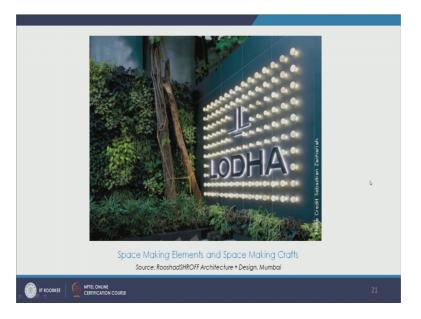
Now, if we look at this in the first instance lot of us would think that these are just bulbs and they are just lit from behind through electric wiring, but that is not. So, these are actually stone bulbs. So, there is a turning machine a turning lathe on which wood turning also happens and then there is a turning machine for stone. So, these are turning machines have been used here to create these stone bulbs and then of course, there are lit.
