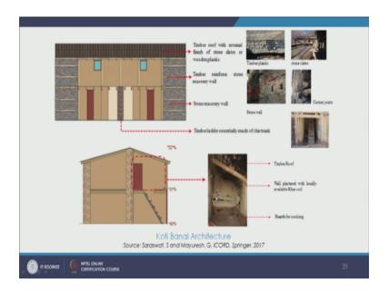
this is village Malari and one residence there and we see the Koti Banal style the alternate timber and stone bands and we see this section over here which shows the spaces this again the interior and the local khar soil and the timber roof over here and we see some corner details and this handmade scooped out staircase.
