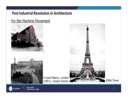
So, here some example of for the machine movement; so, this is crystal palace if you look at the crystal palace, what we were discussing in the form evolved from the structure. And the structural elements are actually the beautifying elements, these are the steel trusses and the steel members which are visible from outside and that is the ornamentation, no other added ornamentation was superficially added.
