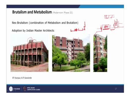
So, if you look at the this is the library building of Kanpur. If you look at the building from outside the structural manifestation of the building is clearly visible, so here in this buildings all these columns and beams are visible through and through or none of the building is hiding the column in the most of the cases if you look at so columns and brick work will blend with each other.
