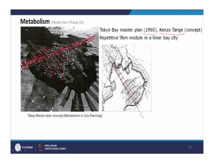
So, here in this Kenzo Tanges concept which is a repetitive 9 kilometer module in a linier bay city. So, this is the line this is the 9 kilometer module which he is designing and this is the services all the services, roads or the infrastructure will be in this access and that is the service- and the servant core and this will be the services which can grow like algae on the water
