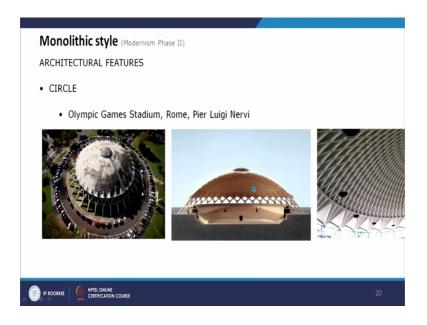
So, this is Pier Luigi Nervis design which is olympic stadium in a Rome so, you can see the structural members and this structural elements are strengthening the roof and Pier Luigi Nervi was Pier Luigi Nervi's other designs are also design emphasize the structure and how structure the structural loads are flowing through the roof and coming as this columns and passing through to the ground.
