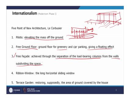
Now, pilotis is elevating the mass of the ground through on a column. So, the ground floor will be something like this, and this top floor will be elevated on the pilotis or the column.
