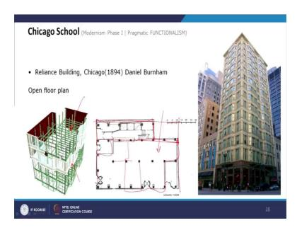
Now, if you look at the system within that so, this is a steel frame structure, from outside we do not see this steel structure because it is cladded from outside. But here this is the
