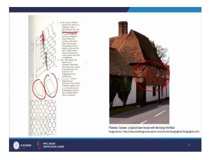
So, another one this is a very quiet common technique when especially with the tiles is the handmade tiles. So, you can see that the same frames you have a small battens going on the horizontal directions and these handmade. So, what you see here is the overlapping of the handmade tiles. So, basically that the tiles are hung on laths or a small battens, which are going so, that to give a triple lap you can see here 1 2 3. So, there is a triple lap each tile covering to others.
