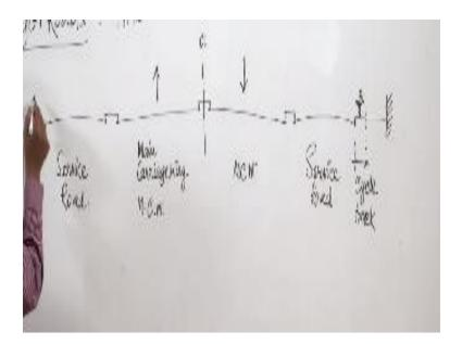
So you can see that this area is kept for cycle track, this is footpath and this is also footpath and this is the median. So this is central line and the median of the whole road section and this is the main carriage where the high speed vehicles like public transportation bus is an all those will go. Basically we keep 11 to 14 meter minimum 14 meter, so that at least 3 to 4 car can go side by side.
