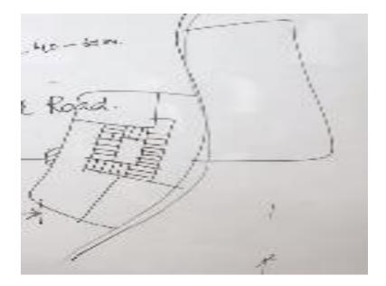
So you can see that that arterial road should have the junction not very frequent very far away junction, but local road they could have junction very near junction because speed of the vehicle in the local roads are less very low than the arterial road.
