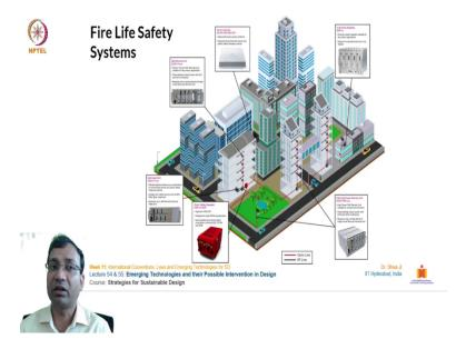
Further there are actually technological interventions in the fire safety also in the buildings. So, new types of actually sensors and isolators are actually coming these days to which can actually sense the fire and can isolate actually a certain segment of the building in order to reducing the spread of the fire in the other sections of the building.
