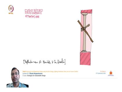
Well traditionally also, how day light strategies have been used you can see in this sketch. So, this window plain is opened to allow the sun at this point of time. And when it is not needed this can be closed and the opening will be closed.
