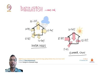
Other dealing with the temperature changes how we can create insulator, the surface insulating material on the envelope of our building to reduce the heat exchange how we can plug the holes and gaps and other leakage points to check the leakage or the fill there are n number of material commercially available in the market today for thermal insulation. So, we must choose them depending upon the uses and application. And while doing so we can minimize the consumption of energy.
