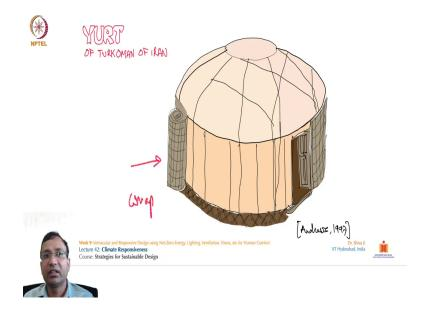
Further if you see how this tribe in Iran has evolved his methodologies of using a different material in different cross section in the different fashion. You see this is rollable mat of these grass and other material which works as a insulator element for covering this building structure.
