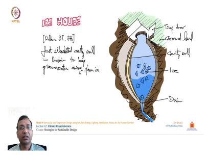
So, how this is used in a several places in the several countries in what ways so, we will discuss with the help of some case examples. So, in this structure if you see the this is the first illustrated cavity brick wall which was found in the country of Britain. And it the cavity wall is kept to keep the ground water away from the ice. So, this is the approach which has been used in this design over here. So, you can see how this is passing from the external side of it.
