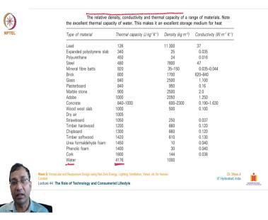
Further on the material part coming down to the material fall. If you see the relative density, conductivity and thermal capacity of the range of materials. So, three things we are talking about here and this is also one of the most important charts and tables for us to be aware of the kind of a materials what we have choosing. And how much of impact these are going to have on our designs.
