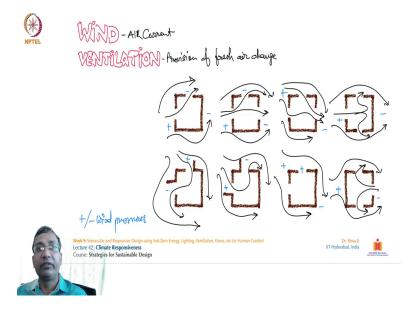
Further to this what could be the other strategies, so ventilation is one of the very important requirements of any buildings. So, how we can plan the openings in our building because there is always some wind. So, how we can even if it is not the wind is not very fast, so how we can create actually high pressure and low-pressure micro zones to induce to the wind inside our premises. So, this slight talks about that, so, how we can promote cross ventilations.
