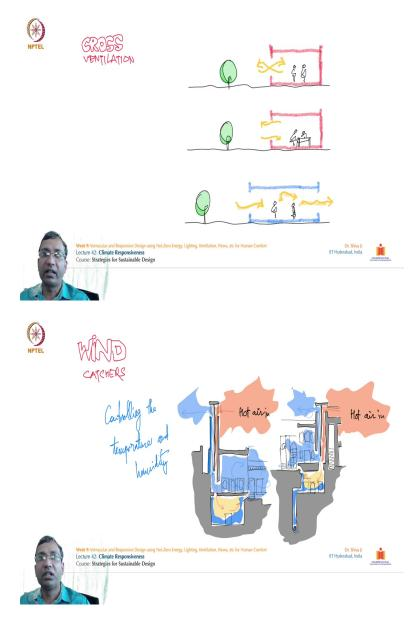
Further continuing our previous discussion. So, in the cross section also, we can plan our openings in such a way the one we saw in this like a wind tunnel wind, breeze wall this cross section. So, similarly we can have even if we are not going to have very tall structures. So, how we can plan the openings the cross section of these openings the length and width of this opening, we can make them vary and depending upon that we can control the passage wind through premises.
