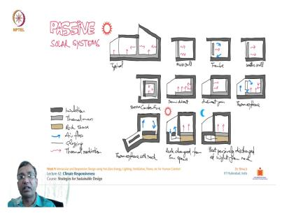
There are several other this, there is a passage solar systems mechanisms which employ the specific materials which we saw in the previous slide embodied energy. And even the conductivity how much of the heat they are going to transfer to the internal quarters. So, depending upon this property we utilize these materials in different combination whether how much of heat we want to allow on interior of that space and how much we do not want to.
