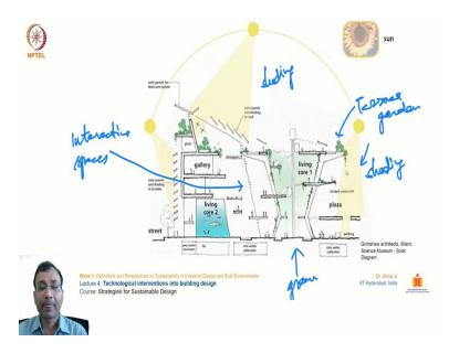
As you can see in this cross section over here of this building, the designer has the architect has utilized the orientation of the sun to maximize the solar gain on the solar panels, as well as reducing the solar gain in the inside of the spaces so that it does not get too heated. At the same time, they have utilized this courtyard designed to create corridors and walking areas along with some greener facilities.
