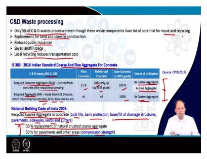
Now, finally, we have to once we collect following the schedule and all we have to design our C and D waste processing and transport plants and all. So, what we find is, after all this we have to actually process the C and D waste. So, in India around only 5 percent of C and D waste is processed, even though because there is lot of a potential for this kind of C and D waste was for reuse and recycling, but still only 5 percent is processed currently, but we have to improve upon it.
