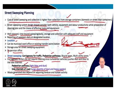
So, then how do I plan for street sweeping the, so, as we have learnt earlier, the cost of street sweeping and collection is very high, and it is higher than the collection from storage containers. That means if a person throws a garbage in a storage container, then it is easy to collect that garbage instead of first cleaning the streets gathering the garbage and then putting it in the container or putting it into the vehicle directly.
