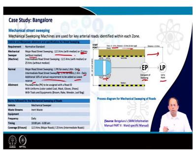
Similarly, for mechanical sweeping also the rate is around 12.5 kilometers with road with medians that means divided roads, because you have to clean from both sides. So, your work doubles almost at 25 kilometers without median. So, you can one vehicle can cover around 25 kilometers if there is no media. So, in addition to that, there is one PK for a Pourakarmika for every one kilometer and major road sweeping is done daily intermediate road sweeping is done daily.
