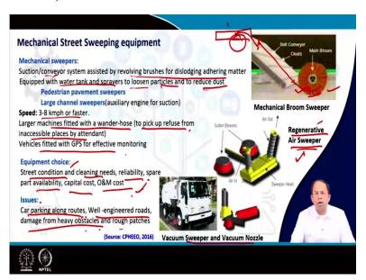
Now, coming to mechanical devices, they can they could be based on either a suction system or a conveyor system. And in both cases, these are assisted by revolving brushes, which the purpose of the brush is to dislodge the adhering garbage from the streets. So, the brushes
