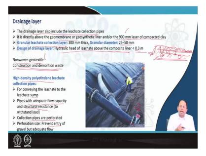
Now, coming to the drainage layer, so, as you can see that you can see these are the liners over here and we have over here the drainage pipes are coming. This is where it is entering into the this particular drainage layer and that so we have got this pipes, the drainage layer also includes leachate collection pipe.
