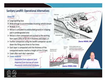
So, next coming to how we should organize our landfill, so, we will talk about the different operational alternatives for the landfill. So, the first method is called an area filled method as you can see, in this particular image, we have a large working face this is the working face of the landfill site. Vehicles can come directly over here and unload the garbage and then machines like this like a bulldozer and all can push the garbage into this particular face.
