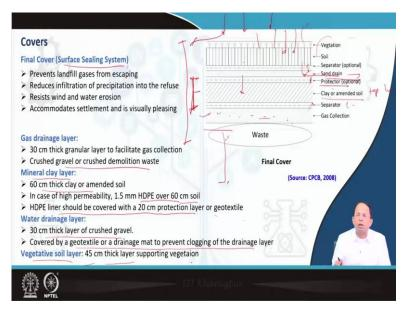
So, this is how the final cover looks like. It is now also known as the surface sealing system. So, we have waste at this layer. Then we have a gas collection layer. Again, it is made of some of gravel. Then there is a separator layer, separator layer could be geosynthetic. Textile, it with some amount of amended soil inside it sandwiched.
