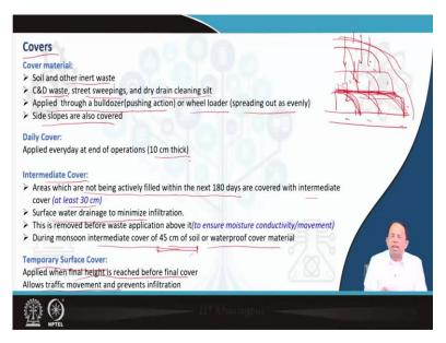
Then comes we have talked about liners which is at the bottom, but we also give sort of liners at the top which we also known as cover. So, we will call them as covers. So, cover material could be either soil and other inert waste, it could be CND waste, street sweeping waste or dry drain cleaning silt with this could be used as the top cover material.
