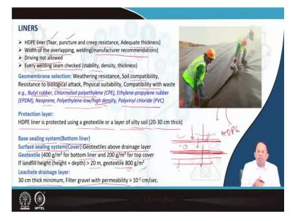
So, as you can see over here, this is that HDPE liner which is being given which has been laid on the top. So, this kind of liners are laid at multiple may be at the top as well. So, usually along with covers also liners are given at the bottom. At the top also, we can have some top liner which is also known as a cover system.
