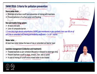
Now, in general, the new landfill design specified by solid waste management rules 2016 talks about prevention of all sorts of pollution. So, first we have to create a proper drainage system for draining the storm water so that, it, we have to prevent it to mix with the leachate. And of course, this will prevent pollution of surface waters and it will allow and during certain rainfall event, there may some amount of flood that happens, so this should be prevented.
