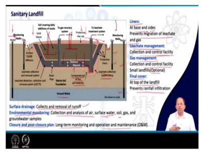
Now coming to a standard sanitary landfill, which is an engineered facility, as you can see in this particular image, it shows the typical sanitary landfill. And here you can see that we have groundwater over here and, and here we are not allowing the leachate to come down and mix with the groundwater, how we have done that. So, you can see here a compacted soil of low permeability is given. So, this is called the liner.
