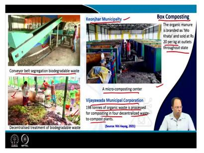
So, over here you can see box composting happening in Keonjhar Municipality over here you can see the boxes, there are some pipes, these are the pipes which are for aeration and this kind of stuff and also some conveyor belt segregation of biodegradable waste. So, some amount of segregation, mechanical segregation is being done using conveyor belts over here and garbage is taken along the belt and some amount of segregation could be done.
