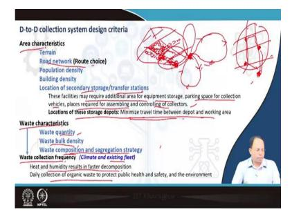
So, first of all the area characteristics plays the largest role, so terrain is important that is what slope, if the slope is pretty steep that means we cannot use hand cuts. So, in that case it is better to go with mechanical vehicles otherwise it is very difficult to push a heavy hand cut with garbage.
