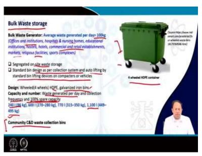
So as you can see that this is a 4 wheeled HDPE container so this kind of container if you will see in many kind of large complexes and also in case of bulk waste generators. So, what individual waste generators we can use smaller containers, but for bulk waste generators, who generate more than 100 kilograms of waste per day we have to obviously use larger containers.
